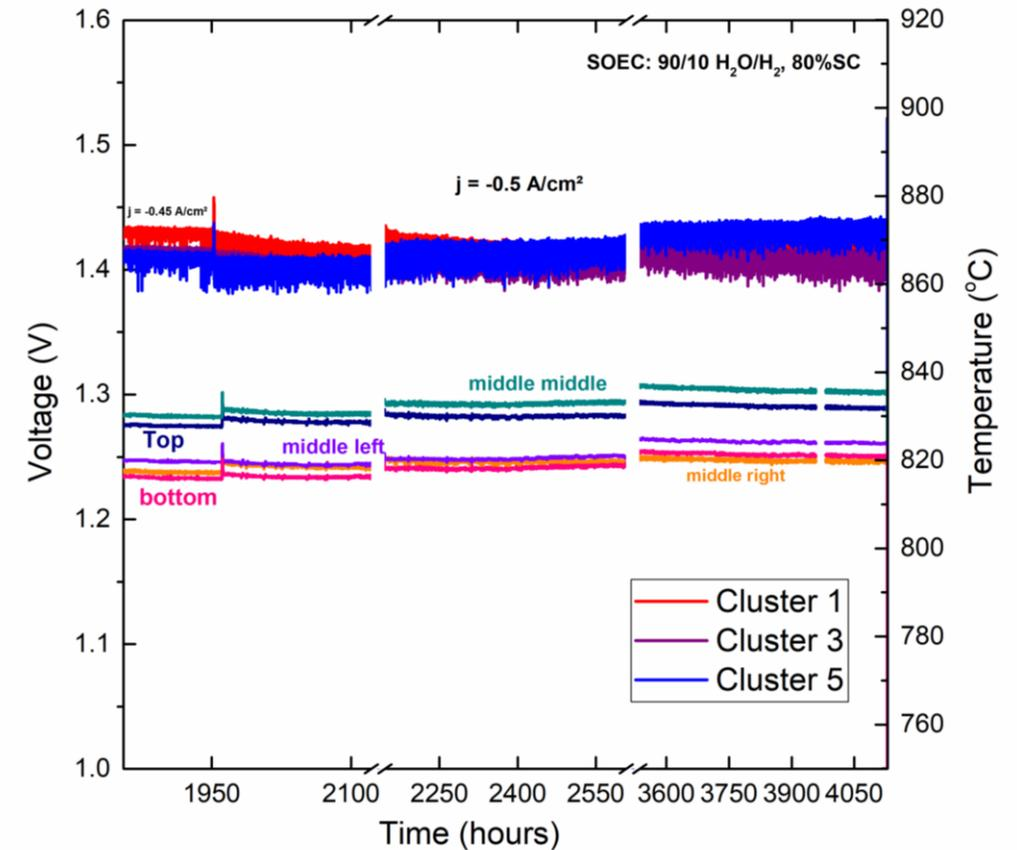
➔ Stack moved to high current density up to  $-0.65 \text{ Acm}^{-2}$
