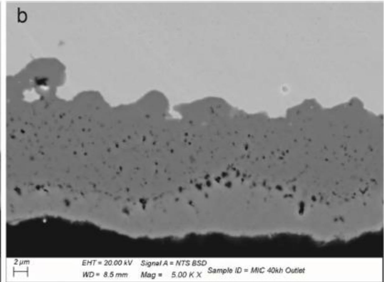
Fuel side, a) center of the stream (850°C, average  $P_{\text{H}_2\text{O}}$ ), b) outlet of the stream (ca. 890°C, high  $P_{\text{H}_2\text{O}}$ )
