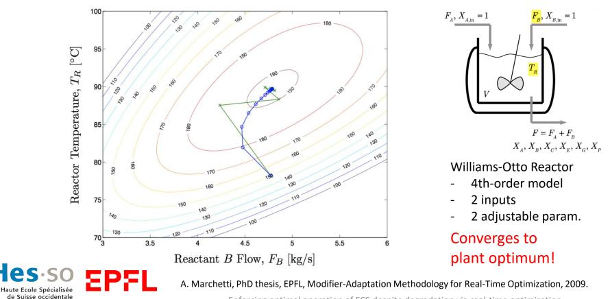
Enforcing optimal operation of FCS despite degradation via real-time optimization
