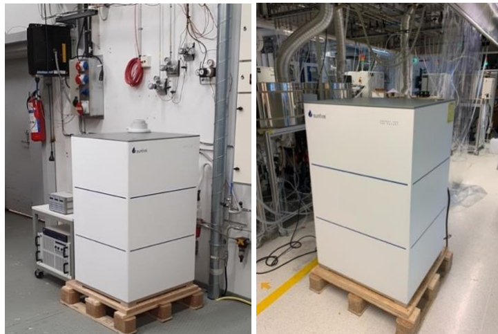
Figure 5 – SOFC \mu -CHP systems for system and stack characterization.
